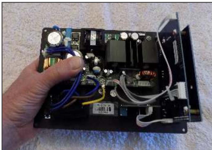
two 250W amp modules and four channels of 24bit 96KHz DSP
